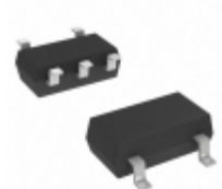
AN80L25RMS Panasonic Electronic Components IC REG LDO 2.5V 0.15A MINI5D
