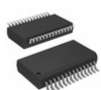
PIC16C57C-20/SS Microchip Technology IC MCU 8BIT 3KB OTP 28SSOP
