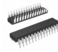
PIC16C57C-20E/P Microchip Technology IC MCU 8BIT 3KB OTP 28DIP
