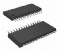
ICL3243CVZ Intersil IC 3DRVR/5RCVR RS232 3V 28-TSSOP
