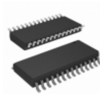
ICL3243CBZ-T Intersil IC 3DRVR/5RCVR RS232 3V 28-SOIC
