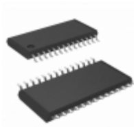
ICL3243CV Intersil IC 3DRVR/5RCVR RS232 3V 28-TSSOP
