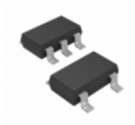
MIC5317-2.5YD5-TR Microchip Technology IC REG LDO 2.5V 0.15A TSOT23-5
