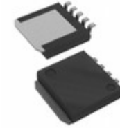
BD3574YHFP-MTR LAPIS Semiconductor IC REG LINEAR 5V 500MA HRP5
