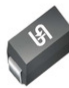
1SMA180Z M2G TSC (Taiwan Semiconductor) DIODE ZENER 180V 1.25W DO214AC
