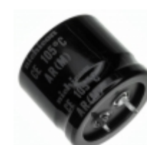
LAR2W221MELB30 Nichicon CAP ALUM 220UF 20% 450V SNAP
