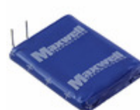
PC10-90 Maxwell Technologies Inc. CAP 10F 2.5V THROUGH HOLE
