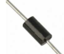
SA78A Fairchild/ON Semiconductor TVS DIODE 78VWM 126VC DO15
