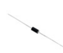
SA78A Littelfuse Inc. TVS DIODE 78VWM 126VC DO204AC
