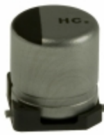
EEE-HC1V100R Panasonic Electronic Components CAP ALUM 10UF 20% 35V SMD
