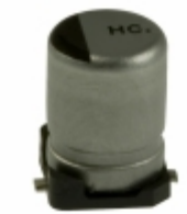
EEE-HC1H1R0R Panasonic Electronic Components CAP ALUM 1UF 20% 50V SMD
