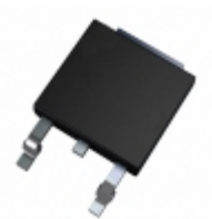
AOD4132L Alpha & Omega Semiconductor Inc. MOSFET N-CH 30V 85A TO252
