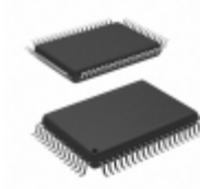
MB89637PF-GT-563-BND Cypress Semiconductor Corp IC MCU 8BIT 32KB MROM 64QFP
