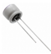
35SVPF39M Panasonic Electronic Components CAP ALUM POLY 39UF 20% 35V SMD
