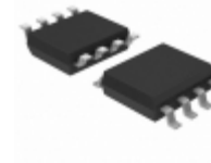
MRF4427R2 Microsemi Corporation TRANS NPN 20V 400MA SO8
