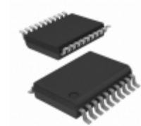
WM8728SEDS/V Cirrus Logic Inc. IC DAC 24BIT STER 192KHZ 20SSOP
