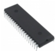
AT89S8253-24PU Microchip Technology IC MCU 8BIT 12KB FLASH 40DIP
