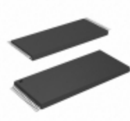
AT29LV020-10TU Microchip Technology IC FLASH 2MBIT 100NS 32TSOP
