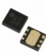
XC6121E628ER-G Torex Semiconductor Ltd IC WATCHDOG TIMER 6-USP
