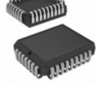
AT27LV020A-90JC Microchip Technology IC OTP 2MBIT 90NS 32PLCC
