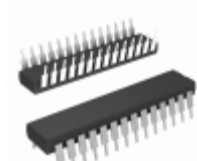
PIC16C57C-20E/SP Microchip Technology IC MCU 8BIT 3KB OTP 28SDIP
