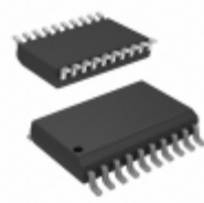
PIC16F1509-E/SO Microchip Technology IC MCU 8BIT 14KB FLASH 20SOIC
