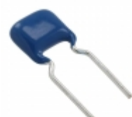
FK22X7R1E156M TDK Corporation CAP CER 15UF 25V X7R RADIAL
