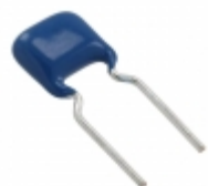
FK22X7R1E226M TDK Corporation CAP CER 22UF 25V X7R RADIAL
