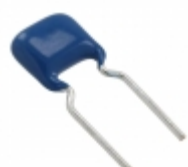
FK22X7R1E106K TDK Corporation CAP CER 10UF 25V X7R RADIAL
