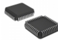
AT27C1024-45JU-T Microchip Technology IC OTP 1MBIT 45NS 44PLCC
