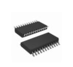
HEF4067BT,653 Nexperia IC MUX/DEMUX 4X16 24SOIC
