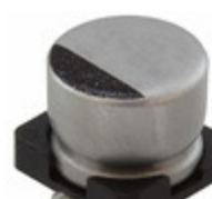
25SEV1000M12.5X16 Rubycon CAP ALUM 1000UF 20% 25V SMD
