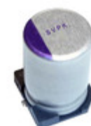
25SVPK120M Panasonic CAP ALUM POLY 120UF 20% 25V SMD
