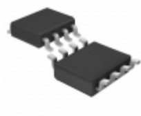
LTC1551CS8-4.1#TRPBF ADI (Analog Devices, Inc.) IC REG SWTCHD CAP INV 10MA 8SOIC
