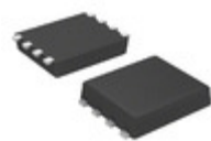
S-1133B49-I8T1U SII Semiconductor Corporation IC REG LINEAR 4.9V 0.3A SNT-8A
