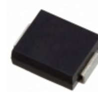
MXL5MCJLCE75AE3 Microsemi Corporation TVS DIODE 75VWM 121VC DO214AB
