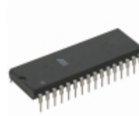
AT27C010-12PI Microchip Technology IC OTP 1MBIT 120NS 32DIP
