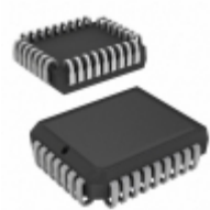
AT27C010-15JC Microchip Technology IC OTP 1MBIT 150NS 32PLCC
