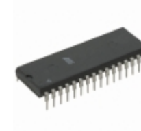
AT27C010-12PC Microchip Technology IC OTP 1MBIT 120NS 32DIP
