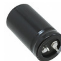
LGR2D471MELZ40 Nichicon CAP ALUM 470UF 20% 200V SNAP
