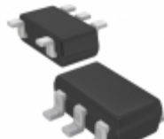
XC6124C429MR-G Torex Semiconductor Ltd IC WATCHDOG TIMER SOT-25
