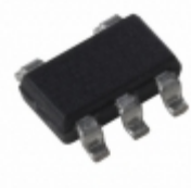
MIC5252-4.75YM5-TR Microchip Technology IC REG LDO 4.75V 0.15A SOT23-5
