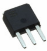
TSM4NB60CH X0G TSC (Taiwan Semiconductor) MOSFET N-CHANNEL 600V 4A TO251
