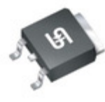
TSM4N70CP ROG TSC (Taiwan Semiconductor) MOSFET N-CH 700V 3.5A TO252
