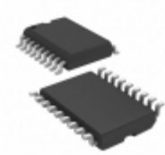
PIC16LC711T-04E/SO Microchip Technology IC MCU 8BIT 1.75KB OTP 18SOIC
