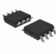
IS25LQ016B-JBLE-TR ISSI, Integrated Silicon Solution Inc IC FLASH 16MBIT 104MHZ 8SOIC
