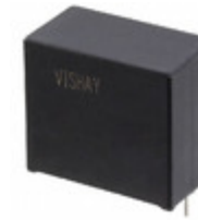
MKP1848C52010JK2 Electro-Films (EFI) / Vishay CAP FILM 2UF 5% 1KVDC RADIAL
