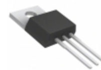
FQP9N25CTSTU AMI Semiconductor / ON Semiconductor MOSFET N-CH 250V 8.8A TO-220
