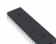
PIC18LC452-I/P Microchip Technology IC MCU 8BIT 32KB OTP 40DIP
