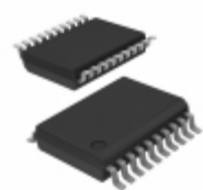
PI49FCT3807DQEX Diodes Incorporated IC CLK BUFFER 1:10 156MHZ 20QSOP
