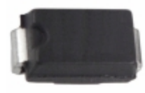
SMAJ75CA-13-F Diodes Incorporated TVS DIODE 75VWM 121VC SMA
