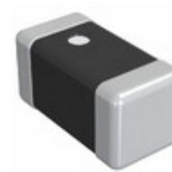
DFE18SANR47MG0L Murata Electronics FIXED IND 470NH 2.6A 54 MOHM SMD
