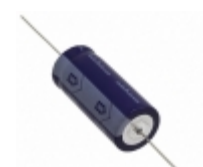
TVX2W101MDD Nichicon CAP ALUM 100UF 20% 450V AXIAL
