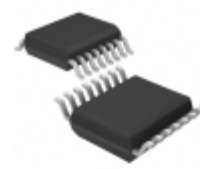
LTC3703EGN#TRPBF Linear Technology IC REG CTRLR BUCK 16SSOP
