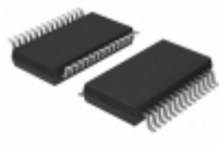
LTC3703EG-5#PBF ADI (Analog Devices, Inc.) IC REG CTRLR BUCK 28SSOP
