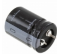
LQS2V151MELZ30 Nichicon CAP ALUM 150UF 20% 350V SNAP
