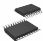
MCP4331-103E/ST Microchip Technology IC DGTL POT QUAD 10K 20TSSOP
