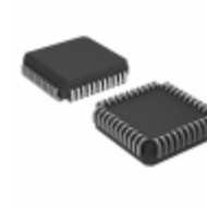
ISPLSI 2032E-225LJ44 Lattice Semiconductor Corporation IC CPLD 32MC 3.5NS 44PLCC
