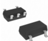
MIC5375-2.8YC5-TR Microchip Technology IC REG LDO 2.8V 0.15A SC70-5
