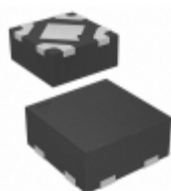
MIC5375-2.8YMT-TR Microchip Technology IC REG LDO 2.8V 0.15A 4TMLF
