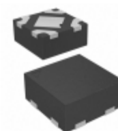
MIC5375-2.8YMT-TZ Microchip Technology IC REG LDO 2.8V 0.15A 4TMLF
