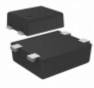
S-80153BNPF-JHETFG SII Semiconductor Corporation IC VOLT DETECTOR 5.3V SNT-4A
