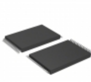
AT49F002N-55VC Microchip Technology IC FLASH 2MBIT 55NS 32VSOP
