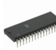
AT49F002N-55PI Microchip Technology IC FLASH 2MBIT 55NS 32DIP
